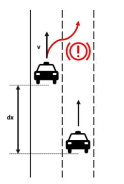
Figure 3: Test scenario for the HiL test
