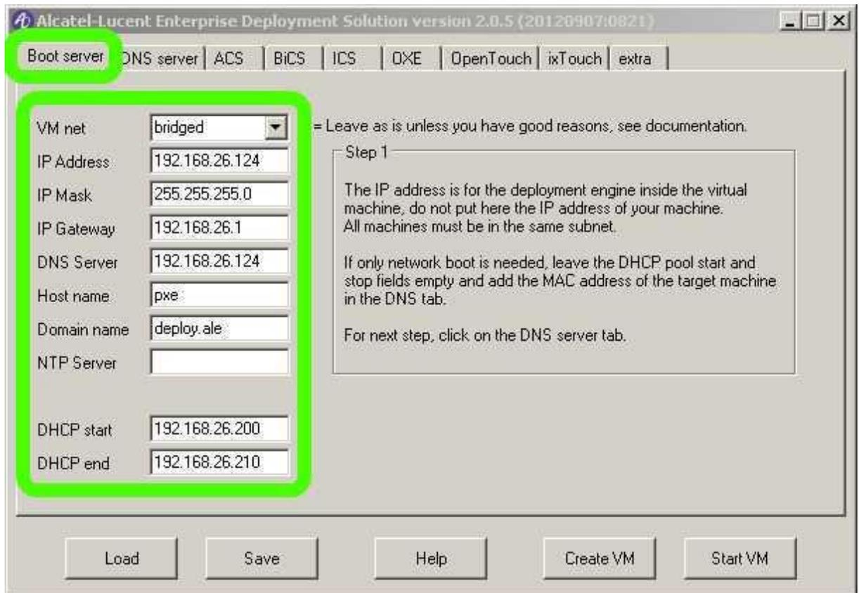
Note that in the "bridged" mode, the Virtual Machine has to be configured to use an IP address fitting the real IP address used by the computer network card.
