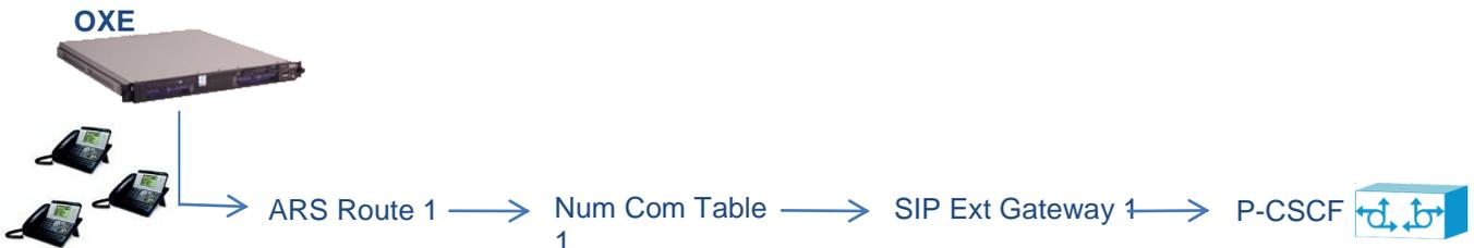
There are 10 steps for On-net calls to Off-net calls. The following chart shows the logic of the configuration of SIP trunk configuration. Steps 1 to 10 describe the call routing mechanisms for public numbering plan. If it's chosen to use a private numbering plan, follow only steps 1 to 8.
